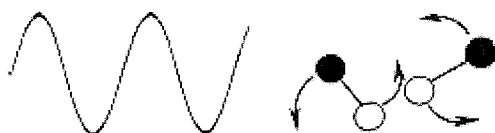
Figure 1.2 An oscillating electric field of appropriate wavelength causes polar molecules to oscillate, generating heat (reproduced from ref. 49 with permission).
