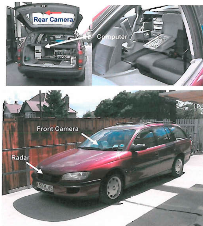
Figure 2.5 TRG Instrumented Vehicle
