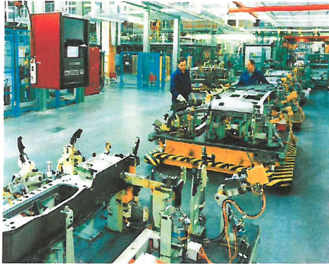
Figure B.2: Manual loading of AGVs.
