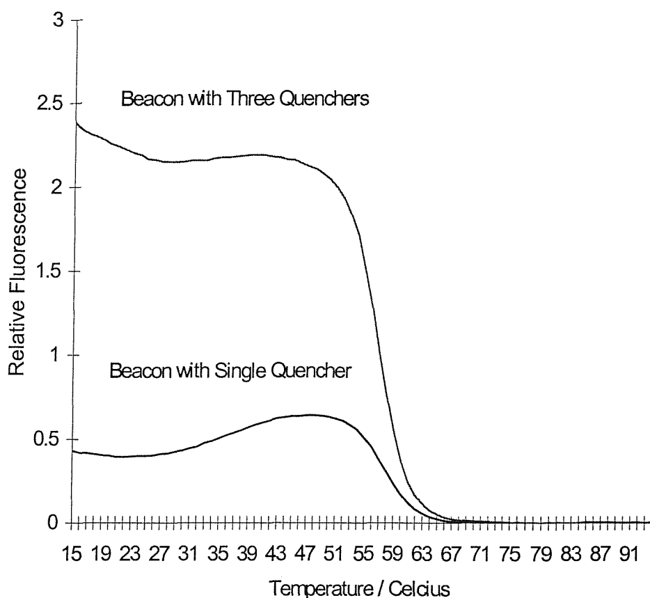
Figure 2.5-6: Fluorescence Melting Curves Comparing Single versus Multiple Quenchers
