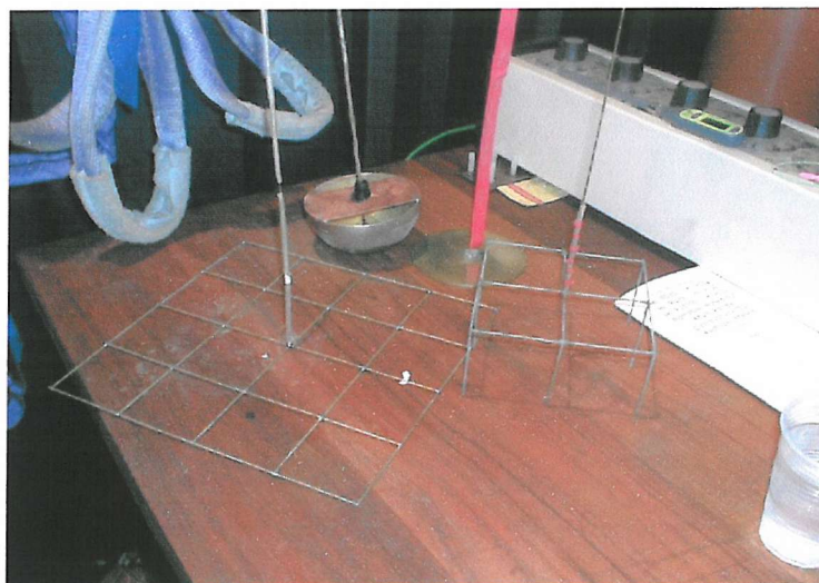
Figure 3.10: Earthing grids 1 – horizontal mesh, combined grid, disc and hemispherical electrode
