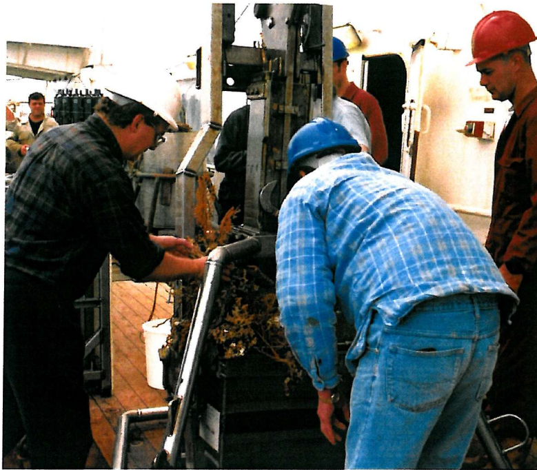
Fig. 2.1 – Box core on the deck of the RRS Discovery during cruise 248 to the Porcupine Seabight. The box core is filled with Lophelia pertusa and associated fauna, and can be seen ‘escaping’ from the top vents
