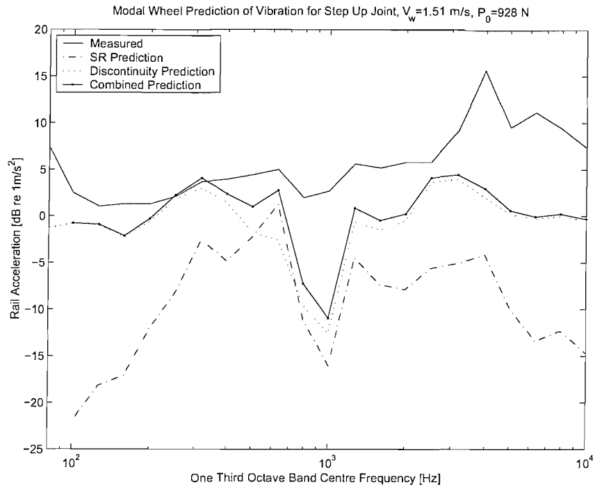
Figure 8–41 Modal wheel variant predicted (with contact filter effects) rail acceleration and measured rail acceleration due to the step-up joint at a wheel pre-load of 928N at a wheel speed of 1.5m/s.
