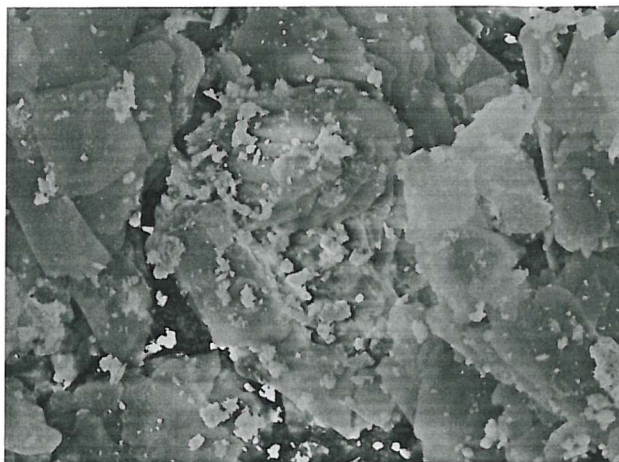
fig. 7.8 a: SEM image of an \text{LaTaON}_2 sample synthesised via solution method (I).
