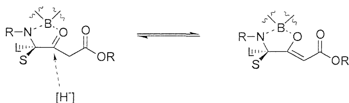
Figure 26. Cyclic transition state models of \beta -keto ester reduction with borohydride.
