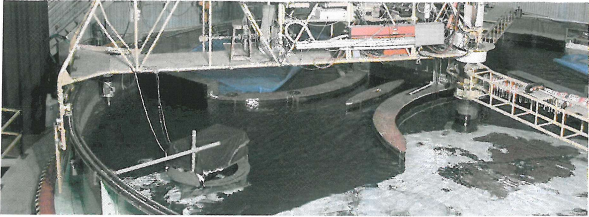
Figure 3.6: Elevated view of the setup in the Coriolis rotating tank. The scanning laser head and mirror were fitted inside the grey box fixed to the tank rim with a steel bar. The observation bridge held the actual laser (connected to the laser head below) and computer acquisition equipment, connected to the camera located above the centre of the channel below. The channel was connecting the two large reservoirs and had a removeable island and barrier.
