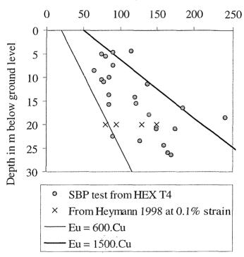
Figure 2.31 Undrained shear strength vs depth for London clay (van der Berg 1999)
