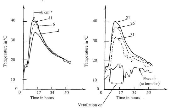
Distance in cm inwards from extrados of 30 cm thick lining
