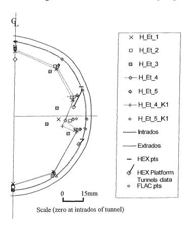
Figure 7.21 Radial stresses in the ground acting on the tunnel extrados
