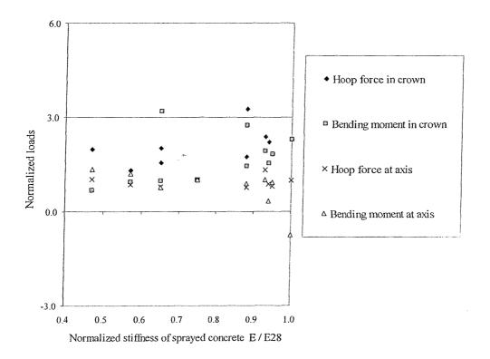
Figure 7.34 Normalized hoop loads vs (RCD/ar)\*(al/r) corrected for tunnel radius and stiffness at ring closure at 9m from the face
