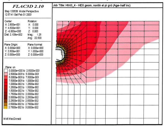
Figure 6.19 Radial stresses in the ground acting on the tunnel lining
