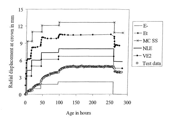
Figure 5.6 Predicted radial displacements at the end of load stage 4
