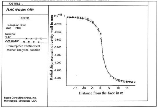
Figure 6.7 Plane strain model for comparison with analytical solution
