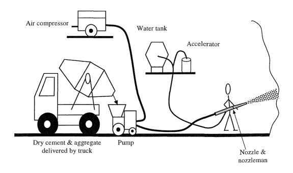
Figure 2.4 Schematic of wet mix (thick stream) spraying process
