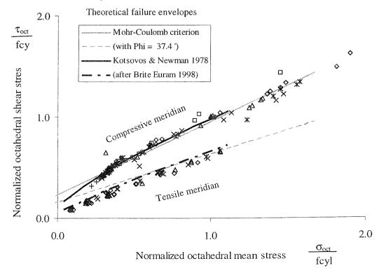
Figure 2.14 Yield stress / peak stress ratio (published data, including data from triaxial tests by Aydan et al. at various confining pressures - sigma 3)
