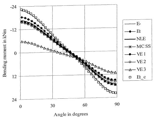
Figure 5.9 Results at the end of load stage 4, normalized w.r.t. model E-(sprayed concrete model = age independent stiff elastic model)
