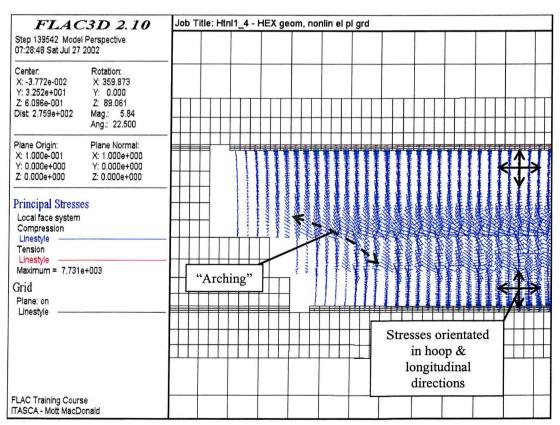
Figure 6.21 Principal stress tensors in tunnel lining - extrados
