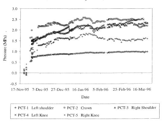
Figure 3.16 Strain gauge measurements from HEX Concourse Tunnel (for locations see Figure 3.17) - Mott MacDonald 1998
