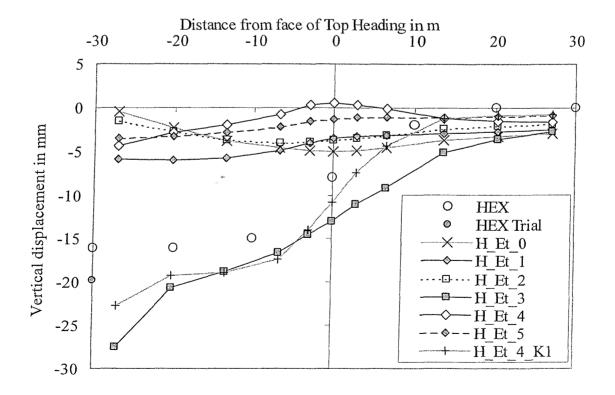
Figure 7.26 Longitudinal movement at 1.5m ahead of the face on the tunnel centreline
