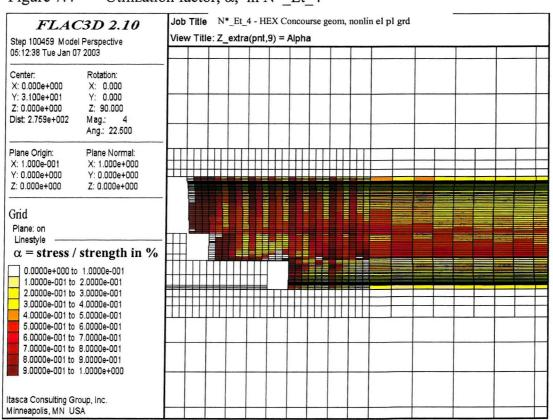
Figure 7.5 Utilization factors at intrados vs distance from Leading Edge
