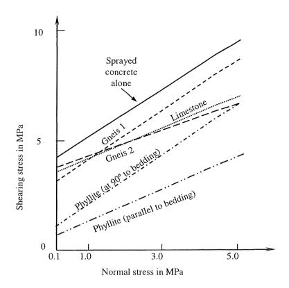
Figure 2..13 Normalized octohedral stress envelope for sprayed concrete (with published data from Aydan *et al.* 1992, Brite Euram 1998 & Probst 1999)
