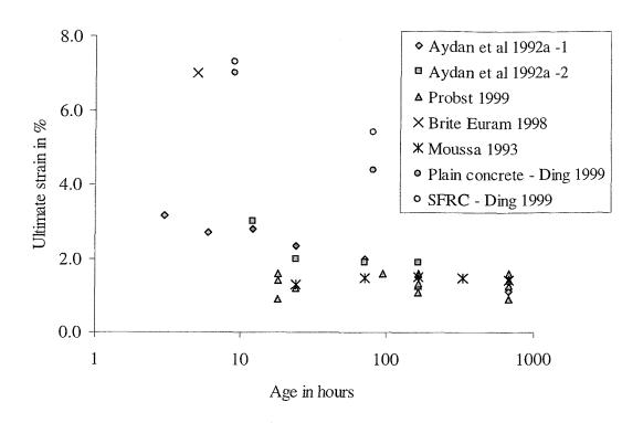
Figure 2.19 Compressive test on sprayed concrete (after Probst 1999)
