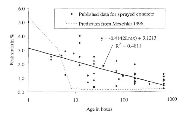
Figure 2.18 Ultimate compressive strain vs age
