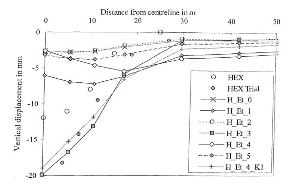
Figure 7.25 Longitudinal surface settlement profile above tunnel centreline
