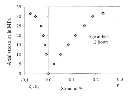
Figure 3.5 Triaxial compressive test on sprayed concrete( $\sigma_2 = \sigma_3 = 1.0 \text{ MPa}$ ) (Brite Euram 1997)
