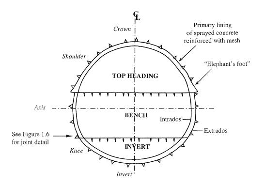
Figure 1.3 Top Heading, Bench & Invert construction sequence
