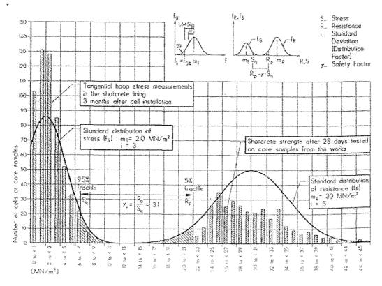
Figure 3.15 Tangential pressure cells from HEX Platform Tunnel at section MMS2 (for locations see Figure 3.17) - Mott MacDonald 1998
