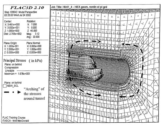
Figure 6.13 Stress paths in ground near tunnel - 0.5m from extrados
