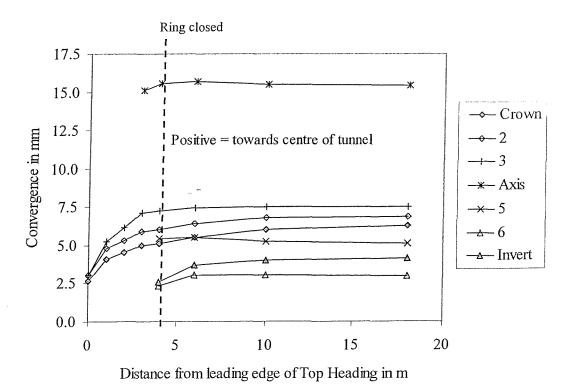
Figure 6.27 Lining deformation 18m from leading edge of Top Heading
