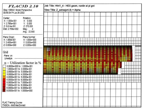
Figure 6.23 Utilization factor in lining - extrados
