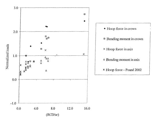
Figure 7.32 Normalized hoop loads vs (AL/R) at 9m from the face
