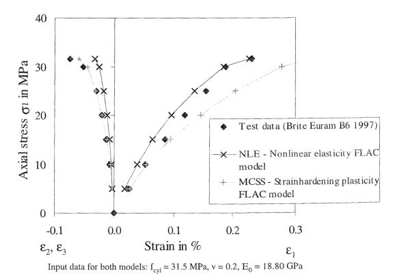
Figure 4.3 Triaxial compressive test on sprayed concrete ( $\sigma_2 = \sigma_3 = 1.0 \text{ MPa}$ )
