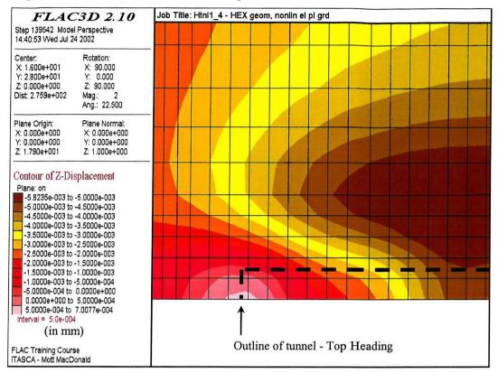
Figure 6.18 Displacement vectors on a transverse plane to the tunnel
