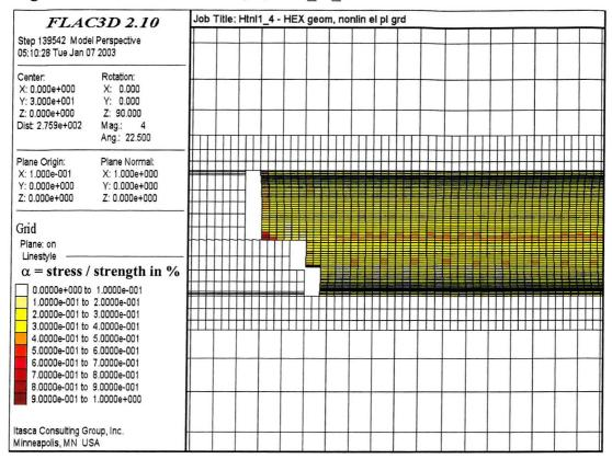
Figure 7.4 Utilization factor,  $\alpha$ , in N\*\_Et\_4
