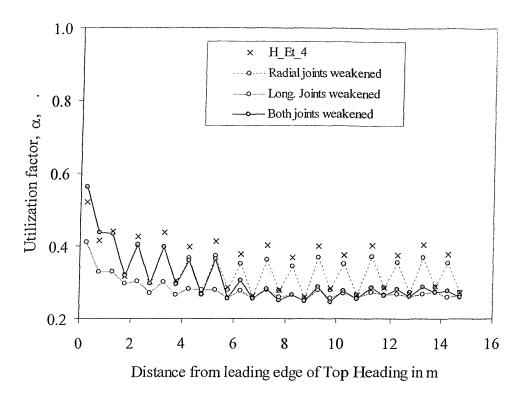
Figure 7.29 Hoop force in crown vs distance from face
