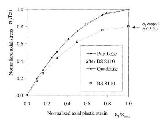
Figure 4.2 Uniaxial compression test on sprayed concrete
