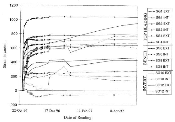
Figure 3.17 Average lining deformations for HEX Platform Tunnels (Mott MacDonald 1998)
