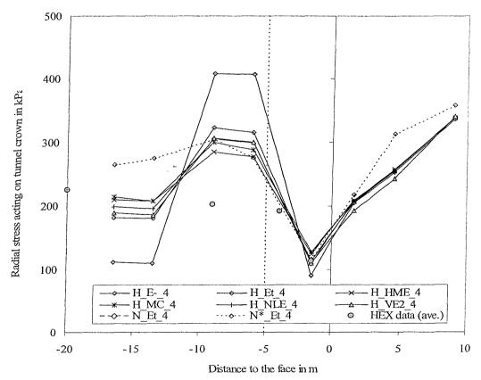
Figure 7.15 Radial stresses in the ground acting on the tunnel extrados
