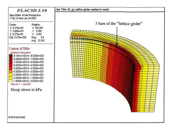
Figure 5.13 The effect of a lattice girder on displacements of the ring (at the end of load stage 4)
