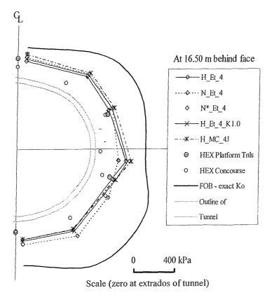
Figure 7.22 Stress paths in the ground near the tunnel extrados – at axis and crown – for different ground models
