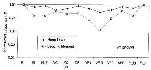
(a) Axial forces & bending moments in circumferential direction at the crown
