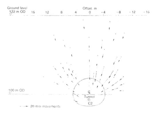
Figure 3.22 Longitudinal movement into the face of the HEX Concourse Tunnel (from inclinometer) - Van der Berg 1999
