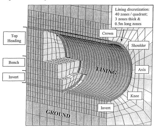
Figure 6.5 Axisymmetric model for boundary conditions study (showing contours of displacement in X direction)
