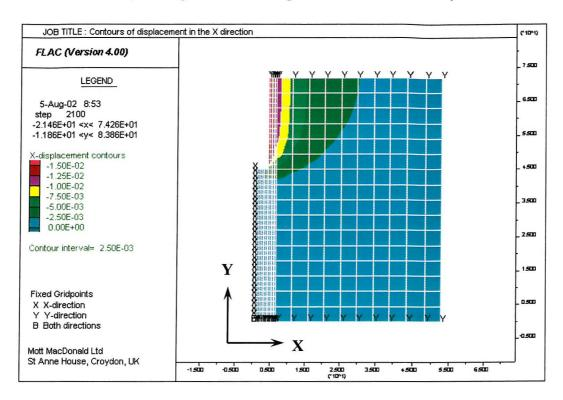
Figure 6.6 Errors in FLAC model w.r.t. CCM analytical solution for axisymmetric model for an unlined tunnel
