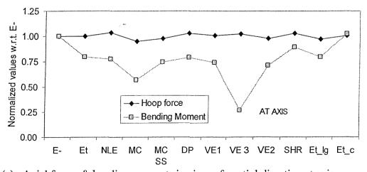
(c) Axial forces & bending moments in circumferential direction at axis
