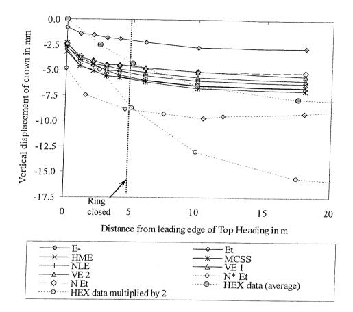
Figure 7.11 Lining deformation at 10m from Leading Edge of Top Heading
