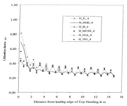
Figure 7.6 Utilization factors at extrados vs distance from Leading Edge
