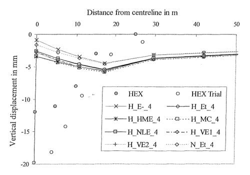
Figure 7.17 Longitudinal surface settlement profile above the tunnel centreline
