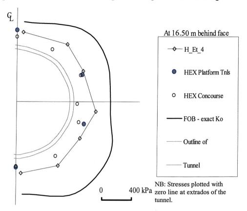
Figure 6.20 Principal stress tensors in tunnel lining - intrados
