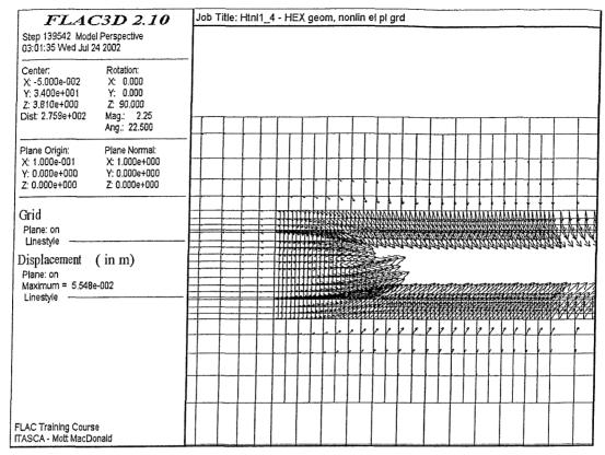
Figure 6.12 Principal stress tensors in ground
