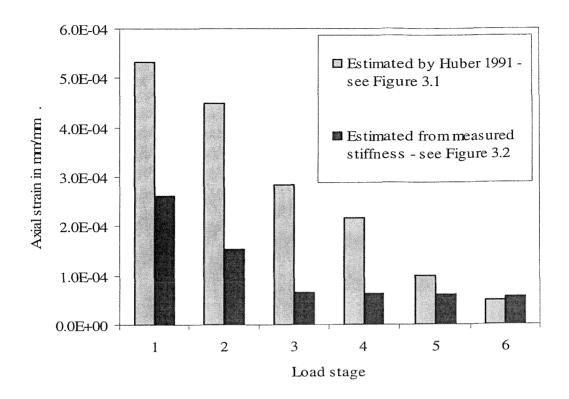
Figure 3.4 Uniaxial compression test on sprayed concrete (Brite Euram 1997)
