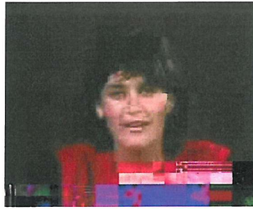
Figure 4.17: Image degradation due to the corruption of DCT coefficient in frame 1, MB83 for the “Miss America” QCIF video sequence encoded at 30 frame/s and 1.15Mbit/s.
