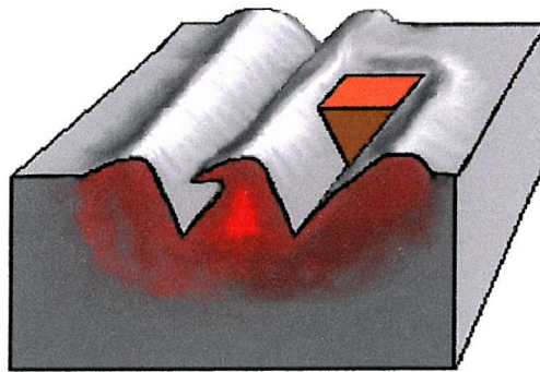
Figure 2.4: Repeated ploughing showing the weakened zone of material [2.22].
