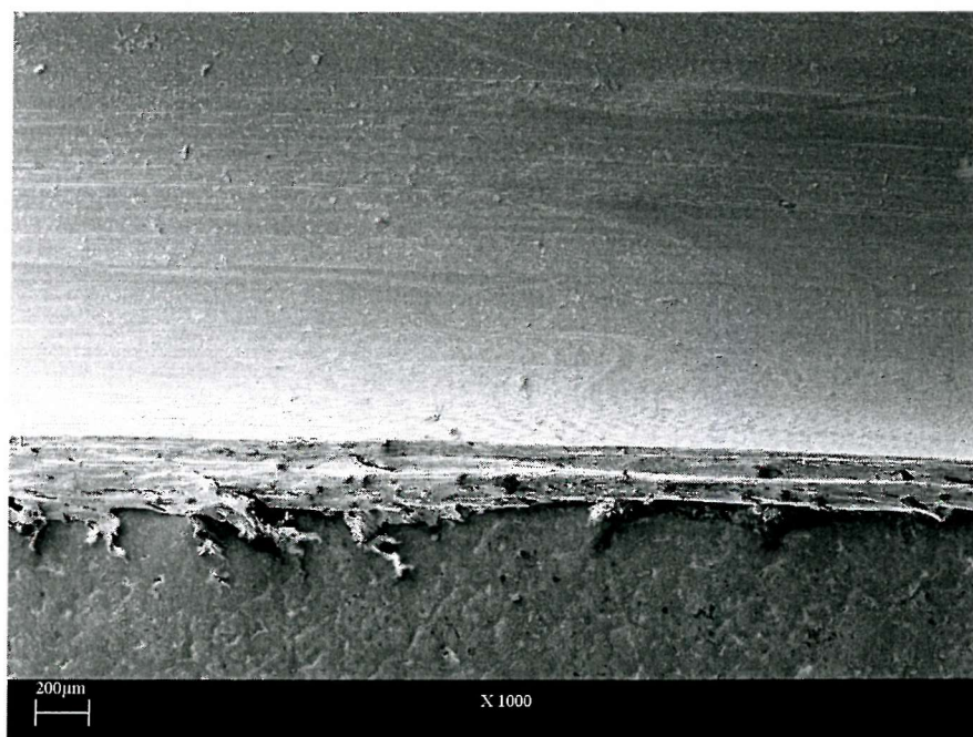
Figure 6.13: SEM image of the PVDF coating showing the edge of the wear track.
