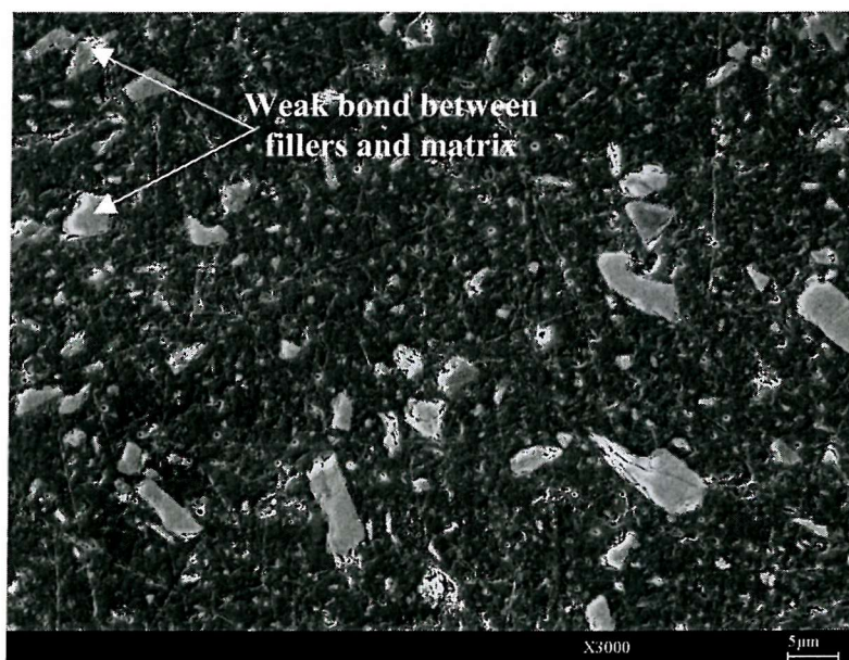
Figure 3.8: SEM of a more detailed transverse section of TS-7.
