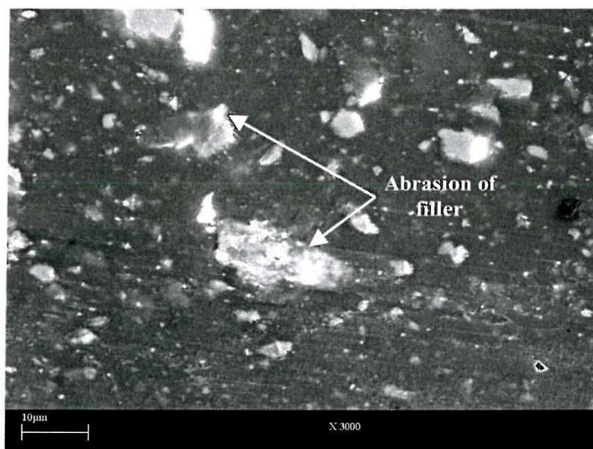
Figure 6.21: SEM image of the worn surface of TS-7. Note the wear of fillers
