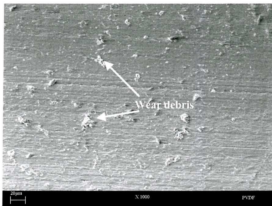
Figure 6.14: SEM image of the PVDF coating showing the centre of the wear scar.
