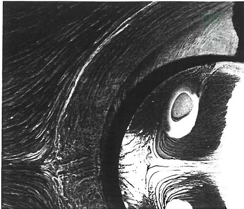
Figure B.3: Surface flow visualisation - flow under horseshoe vortex system, U_\infty = 20\text{m/s} (flow from left to right)
