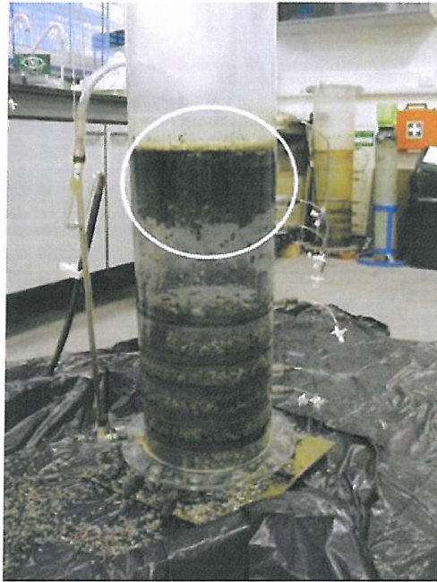
Figure 6-60: Cementation of the top column section (top-2)
