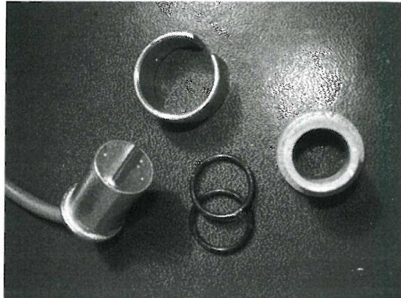
Figure 3.13: Equipment used for inserting bender element probes
