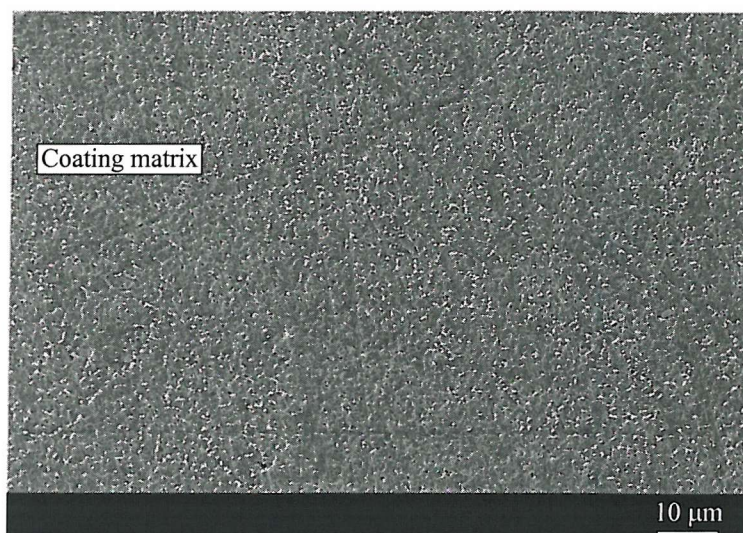
Fig.3.2 SEM image, detail of the matrix of the T-99A coating. Note the structure of this coating is uniform and no particles are in the matrix.
