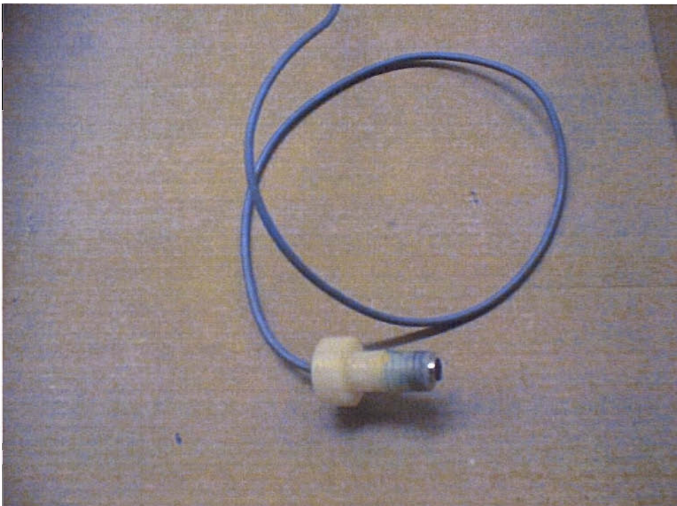
Figure 5.7 Electret microphone with the plastic holder.
