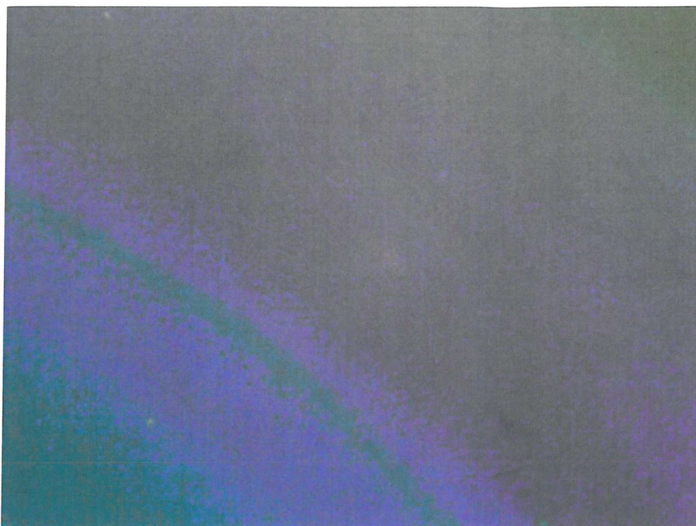
Figure 5.7 One or more blue phases observed in a mixture of 3.42% BDH1281 in 20%/80% FfO-7/9-OfF. The material was in a commercially-made planar cell.
