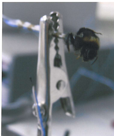
Plate 3.2 A crocodile clip holding the thermocouple measuring the thoracic temperature of the dead Bombus terrestris worker. Note the lower thermocouple used to measure the ambient temperature (picture: James Peat).
