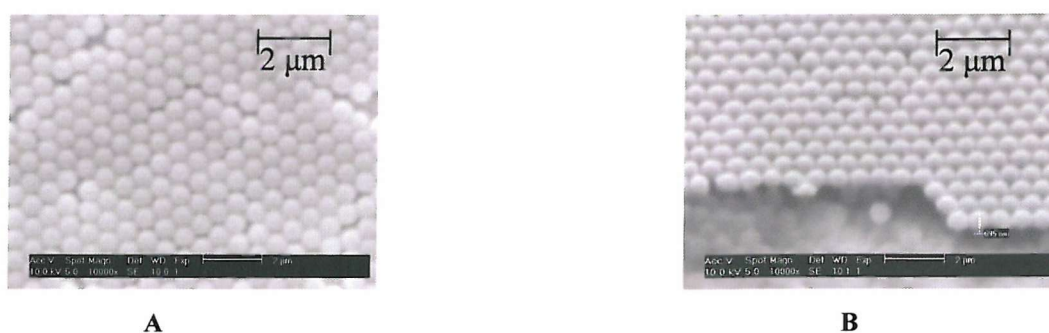
Figure 3.03: Scanning Electron Microscope images of monolayers of 700 nm polystyrene spheres, on an evaporated gold substrate treated with thiol. Figure 3A shows the hexagonal close packed order of the sample, and figure 3B shows the edge of the same sample as viewed from an angle of 30^\circ .
