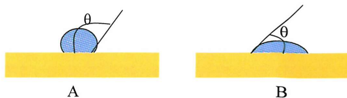
Figure 3.01: Schematic diagram showing the difference in contact angle of water on (A) evaporated gold, and (B) evaporated gold modified by the addition of a monolayer of cysteamine
