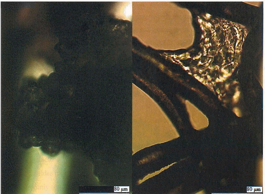
Figure 1.4: Magnified images of an absorbent particle (left) and of its non-woven backing fabrics (transmission mode).
