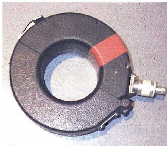
Photo 3.2, A clamp-type RFCT (Radio Frequency Current Transducer)
