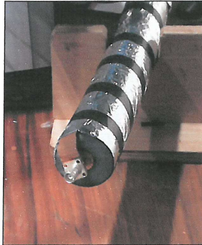
Figure 5.2 – 33kV Cable With BNC Connector
