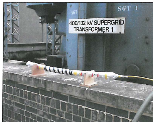
Figure 5.5 – Screened Cable Connected to Oscilloscope
