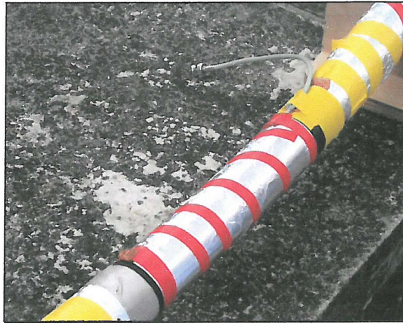
Figure 5.7 – Unscreened Capacitive Coupler with BNC Connector Output
