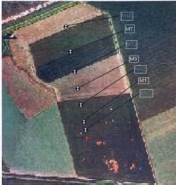
Figure 3.12 Aerial picture of the test site. Receiver locations are shown in black and white with its respective reference numbers and the source is pointed with a red cross.
