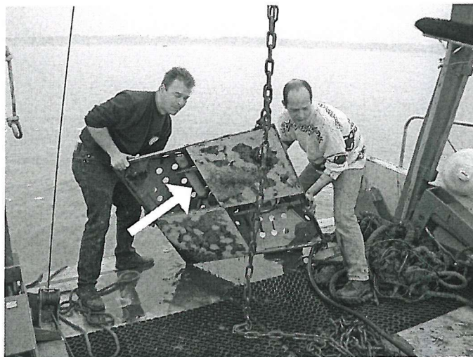
Figure A.3: View of the bottom of the ADCP frame during recovering. White arrow shows the C-T logger attached in the frame.
