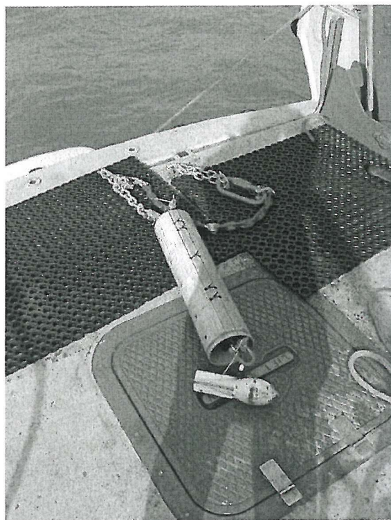
Figure A.4: The surface C-T logger, showing the case, the chain and the weight.
