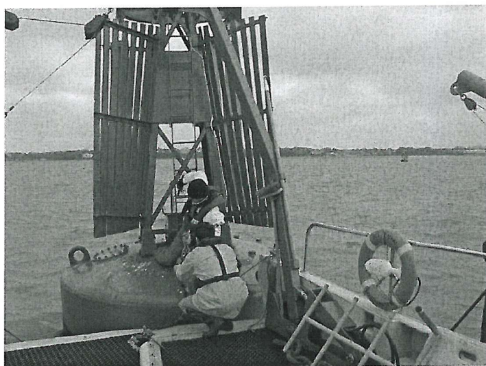
Figure A.5: Attaching the surface C-T logger on the eye of the Cadland Buoy from the stern of the boat.
