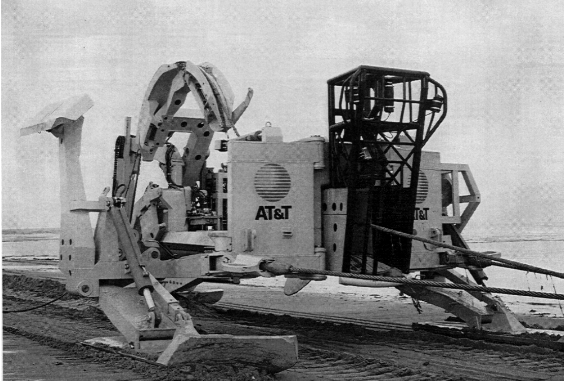
Figure 2 The 4 m long 'Sea Plow VI' towed underwater vehicle can bury cable to a depth of 1.1 m in the seabed at a maximum sea depth of 1 000 m. (From ROV Review 1993-94, WAVES magazine, Windate Enterprises Inc., 5th Edition.)
