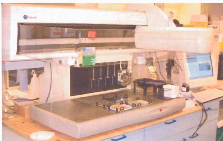
Figure 2.5 – The ‘Perkin Elmer Multiprobe II’ robotic liquid handler, used in automated electrode preparation of composite electrodes.
