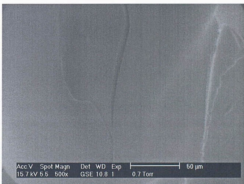
Figure 4.35 - An SEM micrograph of \text{LiFe}_{0.9}\text{Ni}_{0.05}\text{Co}_{0.05}\text{PO}_4 prepared on the high-throughput array – sample B2.
