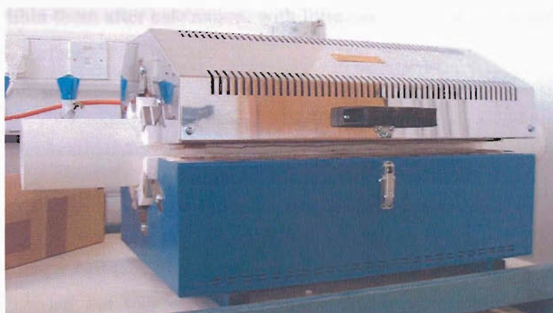
Figure 4.5 - 80 mm large bore tube furnace for combinatorial synthesis.
