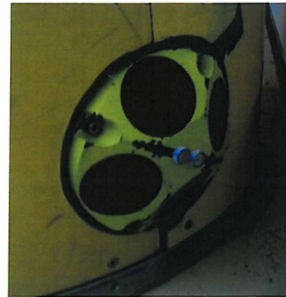
Figure 2.7.2 ADCP fitted to hull
