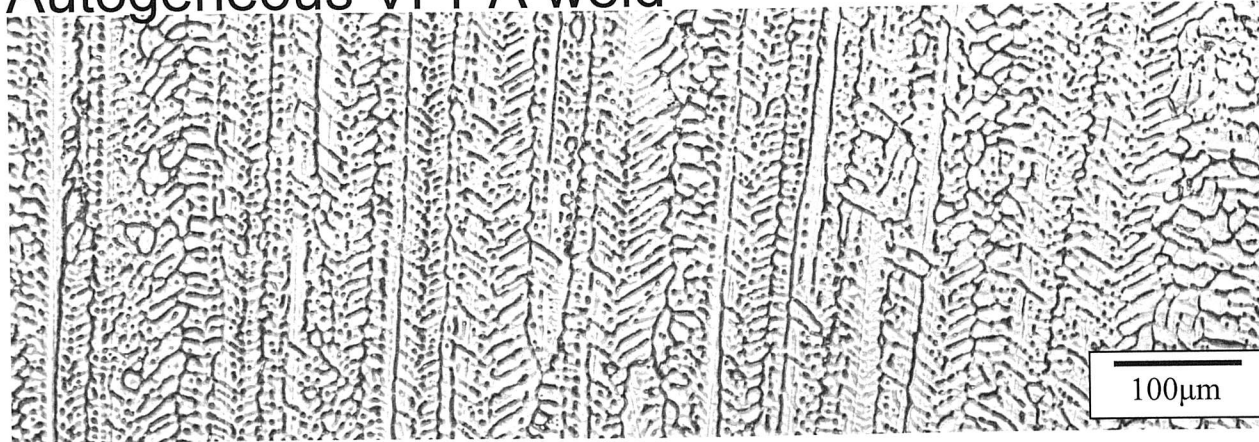
Figure 4.15 Variation of the microstructure in the centre of the fusion zone for the filled VPPA weld (equiaxed structure) and autogeneous VPPA weld (axial columnar)
