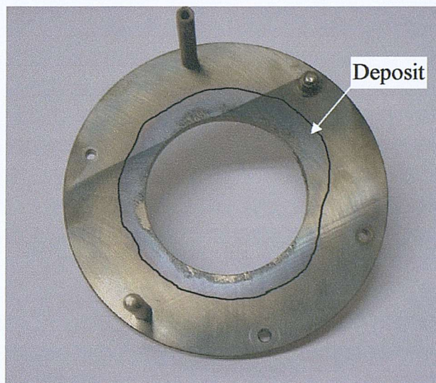
Figure 6.37: Photograph of anode with area of deposit indicated
