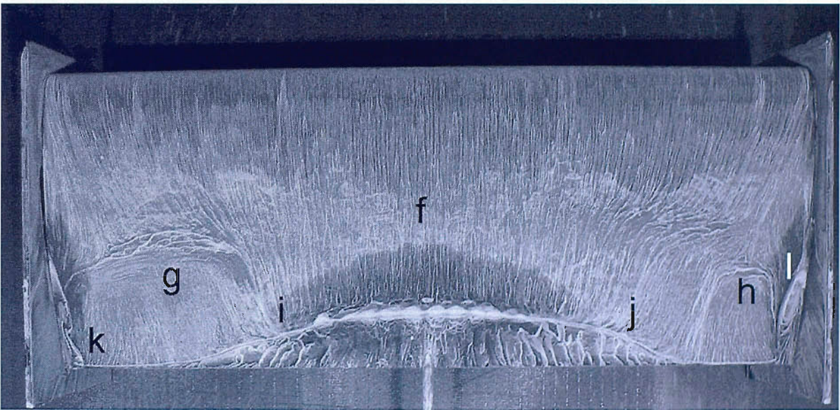
Figure 4.14: Suction surface flow for the wing in ground effect at h_r/c = 0.153 and 5 deg aoa, while behind the upstream wing and bluff body.
