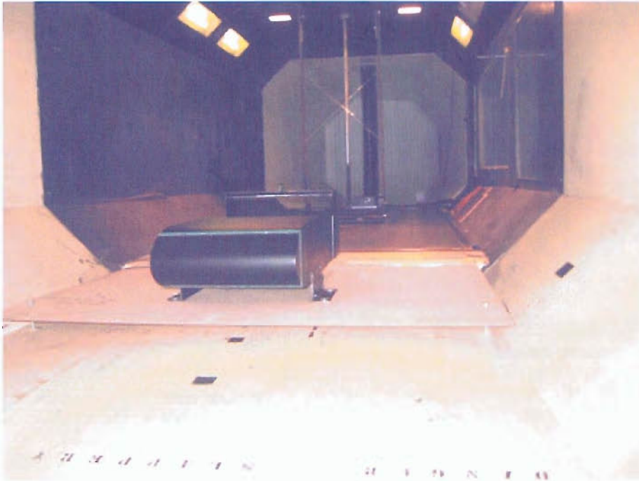
Figure 3.4: The diffuser bluff body and associated ground board that were used in the experimental tests.
