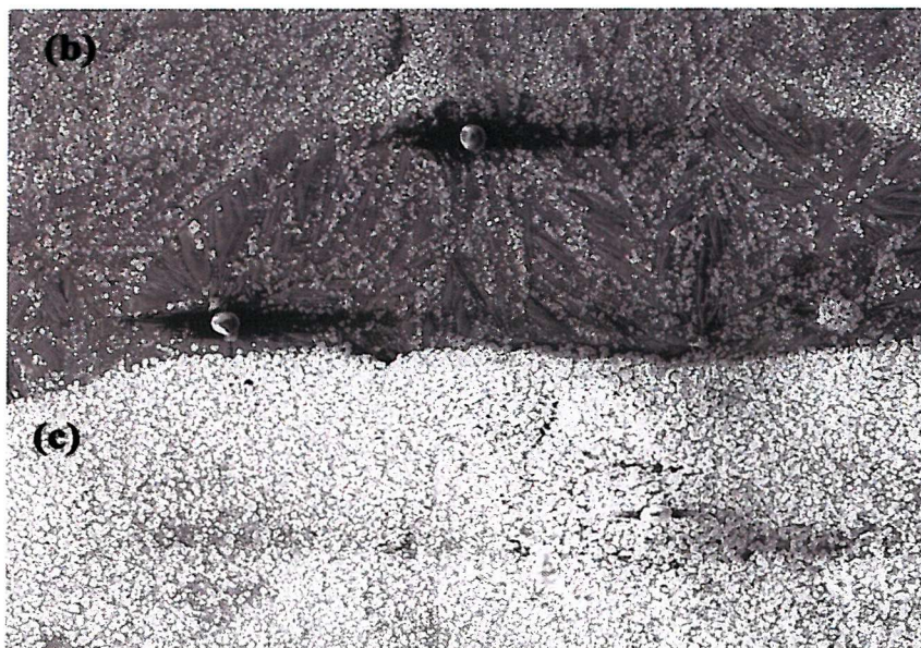
Figure B.2: SEM picture of the damage of a sample due to annealing. The picture is taken from the edge of the sample where maximum damage occurred. Region (c) suffered more damage than region (b) as it is close to the edge. (See also Fig. B.1)
