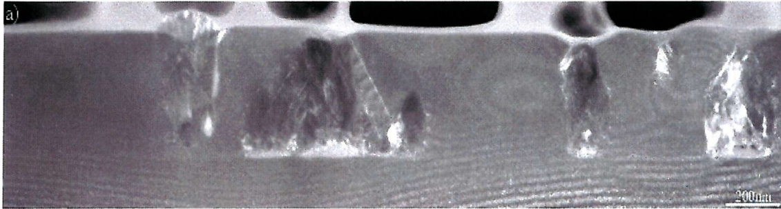
Figure C.2: TEM image of epitaxial germanium grown using Molecular Beam Epitaxy. Starting with germanium wafer as substrate \sim 375 \text{ nm} thick layer was grown at 275^\circ \text{C} . The image shows cross-sectional view of the growth related defects.
