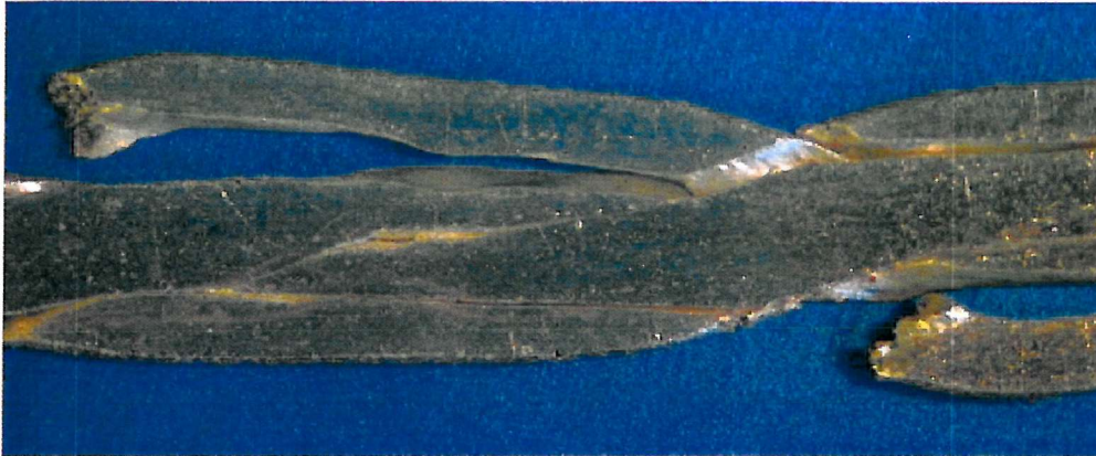
Fig. 70: Braided wire broken by the shear stress produced on the transposition of the external wires when the rolling plane is turned 45^\circ .
