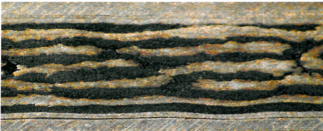
Fig. 25: Longitudinal section of a burst wire of \phi=3,46\text{mm} .
