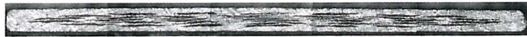
Fig. 29: Standard tape rolled in a single step from 500 \mu\text{m} to 190 \mu\text{m} with a further rolling at 170 \mu\text{m} . (width=3.70 mm).
