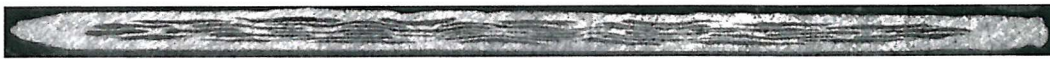
Fig. 28: Tape rolled between copper tapes of the same overall size with a further standard rolling of the tape to 170 \mu\text{m} (width= 4.64 mm).
