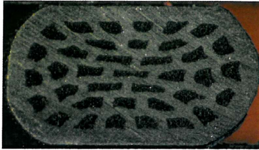
Fig. 14: A tape with 37 filaments of Au-Ag alloy (10%), rolled in the first steps at 100 \mu\text{m} ratio per pass.
