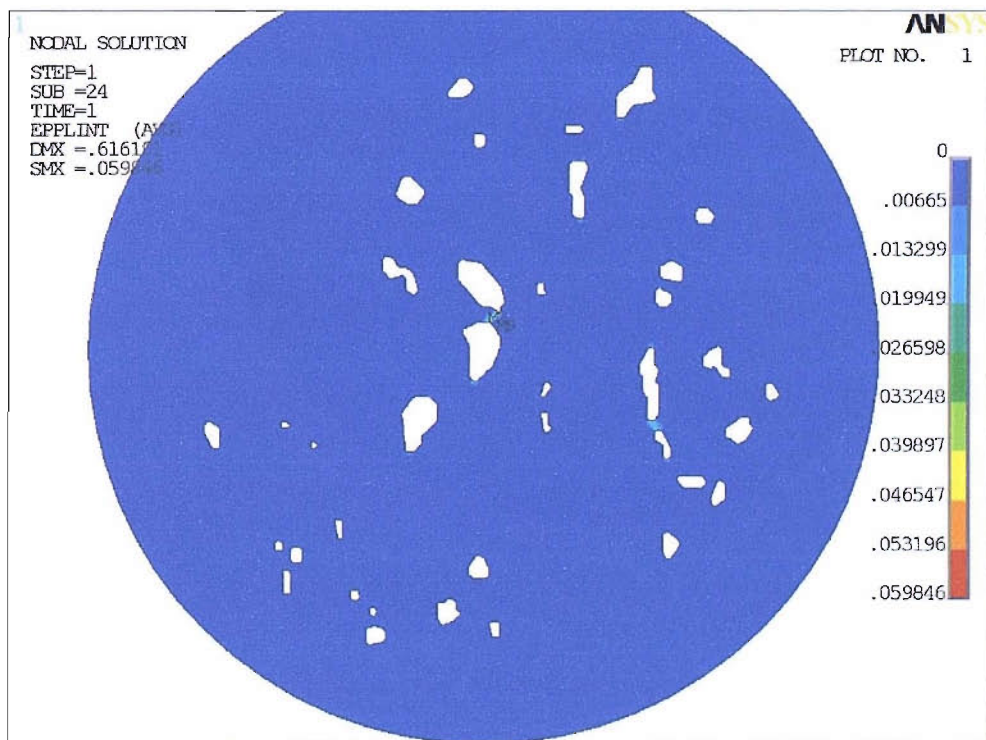
Figure E-2 (a): Maximum plastic shear strain within Al matrix for Area 3
