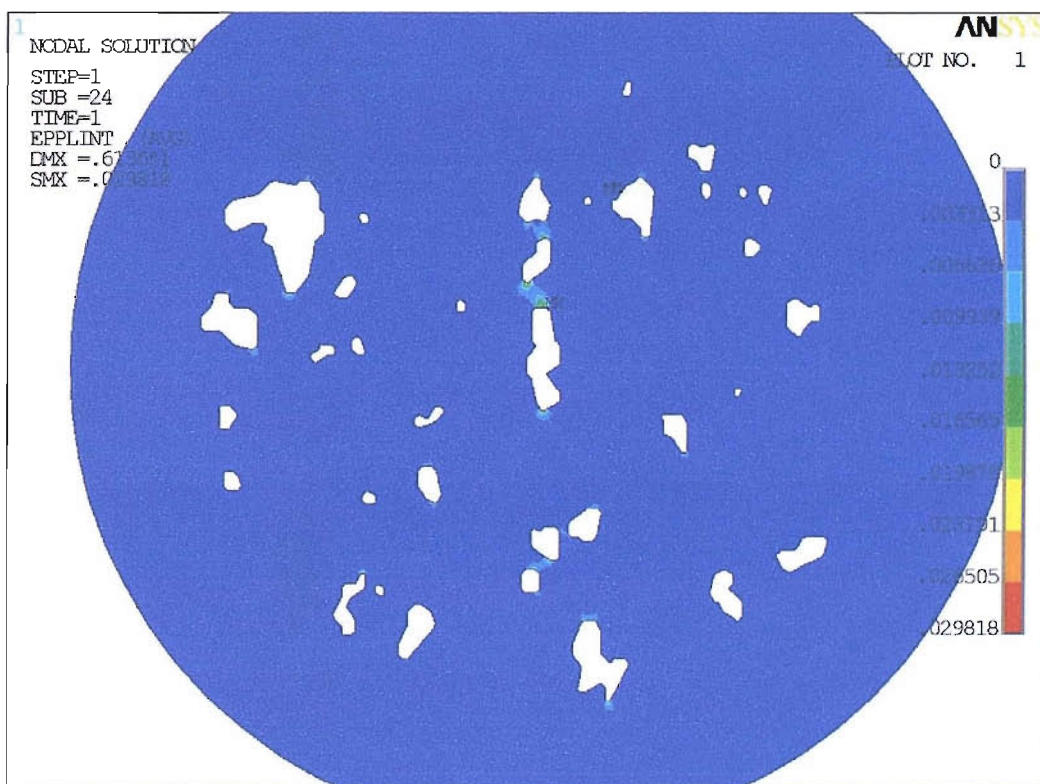
Figure E-1 (a): Maximum plastic shear strain within Al matrix for Area 1
