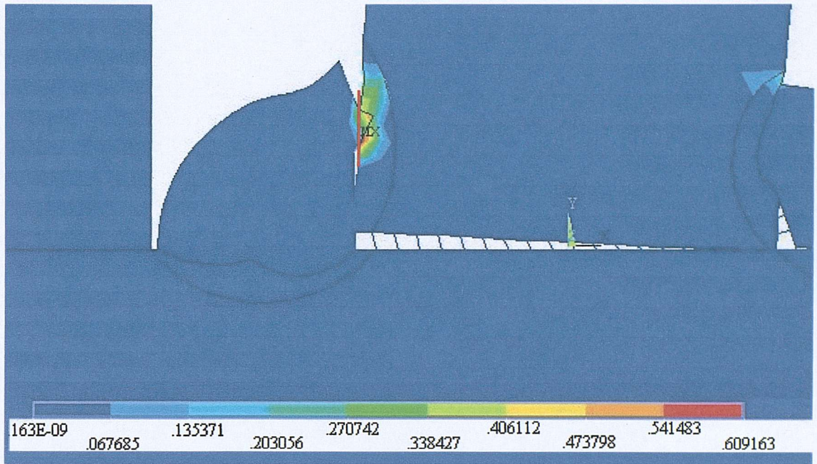
Fig. 7-13 Total von Mises strain distribution of model WT1-B for an applied displacement of 3 mm
