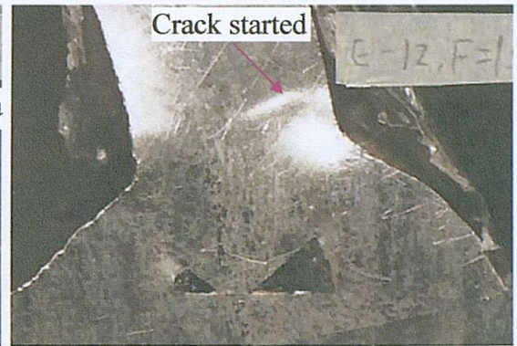
(b) Crack emerged and propagates at the attachment plate
