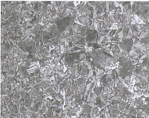
(e) Microstructure in the transition area from HAZ to weld metal, \times 500
