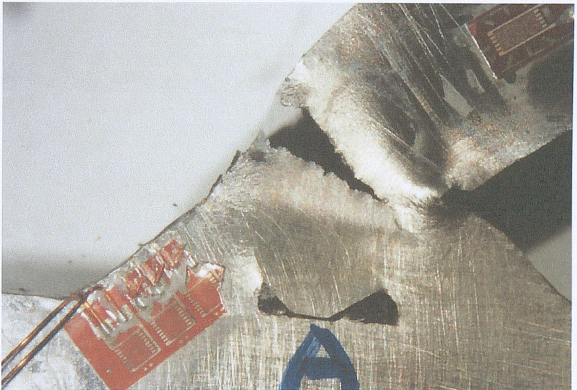
(b) Specimen failed through the plate (Specimen A)
