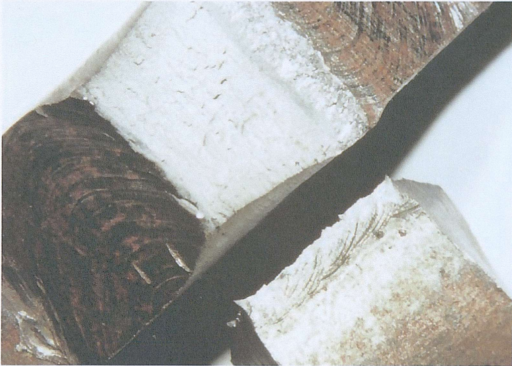
Fig. 5-30 A typical failure surface of the WT2 bending specimens
