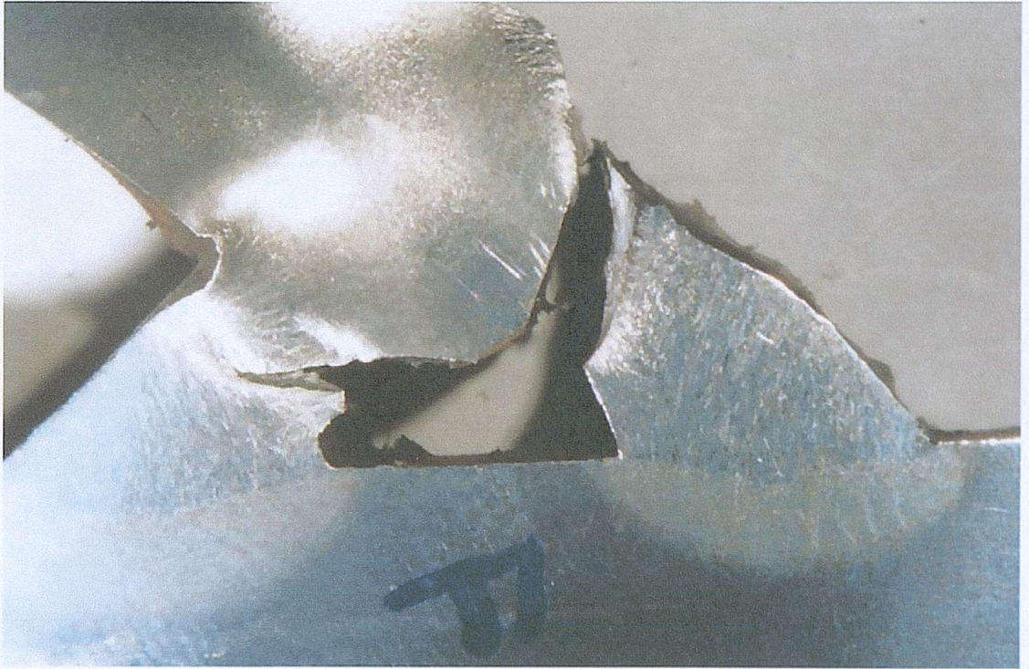
(a) Specimen failed through the weld (Specimen F)
