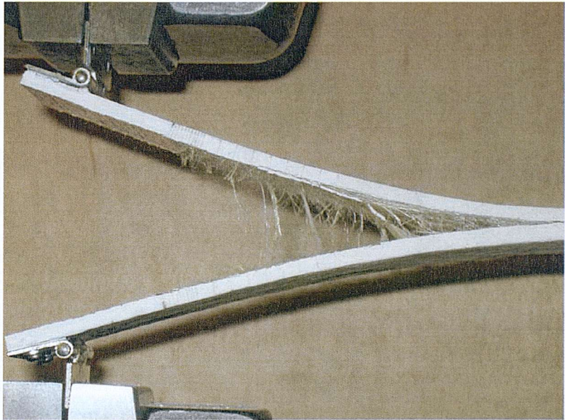
Figure B.1: Fibre bridging at a Kevlar/E-Glass/Ampreg 75 specimen whilst loaded in opening mode
