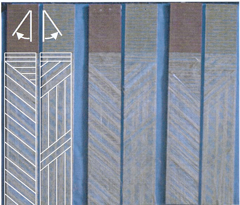
Figure B.10: Interfaces of three Kevlar/E-Glass/Ampreg 26/75 specimens
