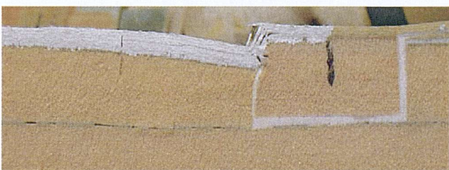
Figure 6.7: Load-failure mode sequence for Sample Rp. 6 subjected to 779J blunt object impact.
