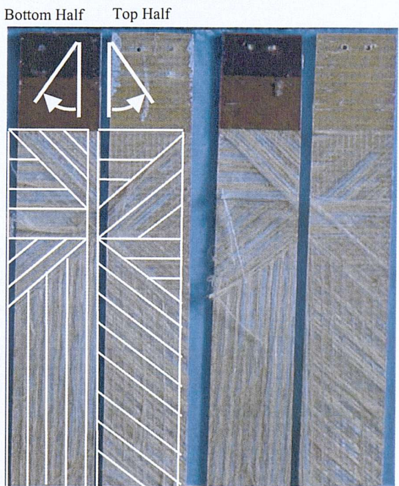
Figure B.4: Interfaces of two typical Group A Kevlar 75 specimens after complete failure
