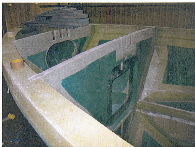
Figure A4: Bulkhead joints in bow section of Trent Lifeboat
