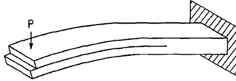
Figure 4.10: Loading configuration of the ELS test method
