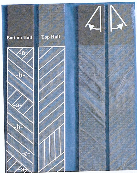
Figure B.7: Interfaces of two typical Kevlar/E-Glass/Ampreg 26 specimens
