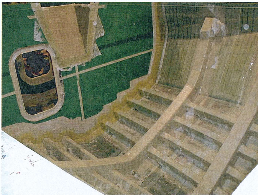
Figure A5: Stiffening arrangement within the hull of a Severn class lifeboat
