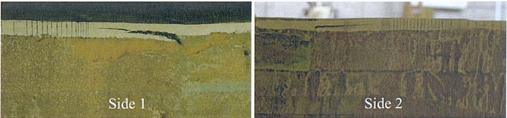
Figure 6.12: 1270J impact damage sustained by Specimen Rp.19
