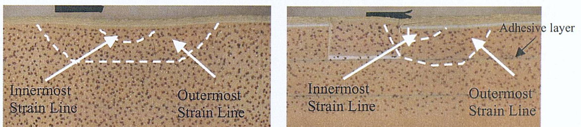
Figure 5.11: Strain line formation in PVC foam in pristine and repaired beams viewed by the stereoscopic photographic NDE technique
