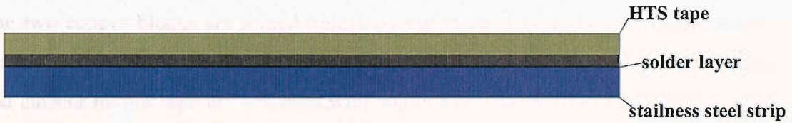
Figure 5.9. Schematic of the longitudinal cross section of the HTS tape sample soldered on the steel strip
