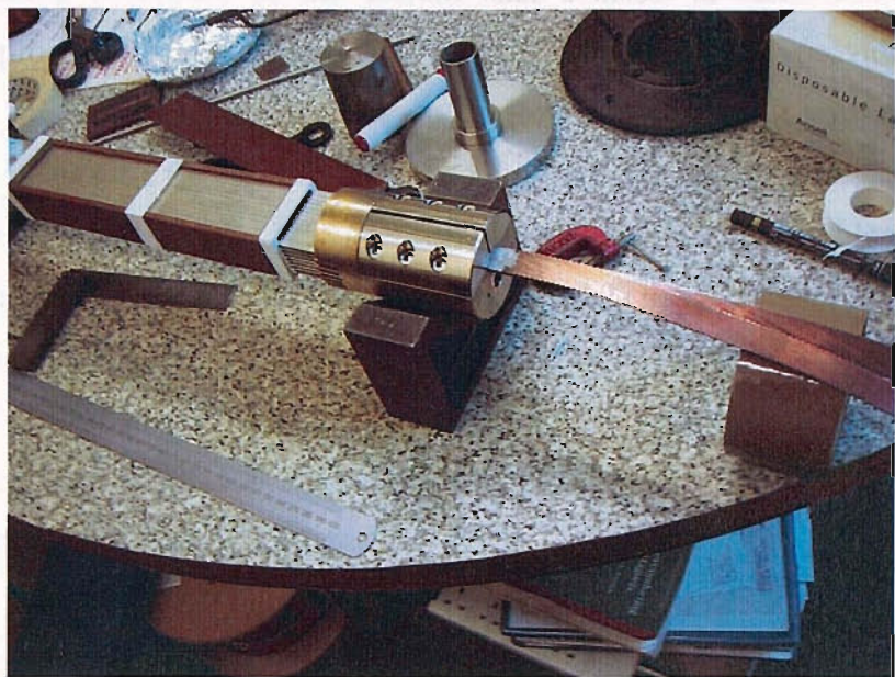
Figure 3.25. The HTS part with the LTS Rutherford cable soldered in the 4.2 K terminal
