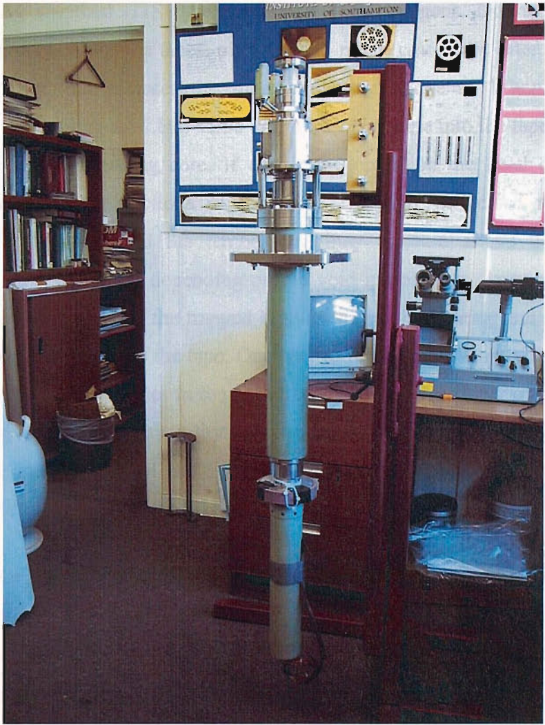
Figure 3.31. The 7.5 kA current lead ready
