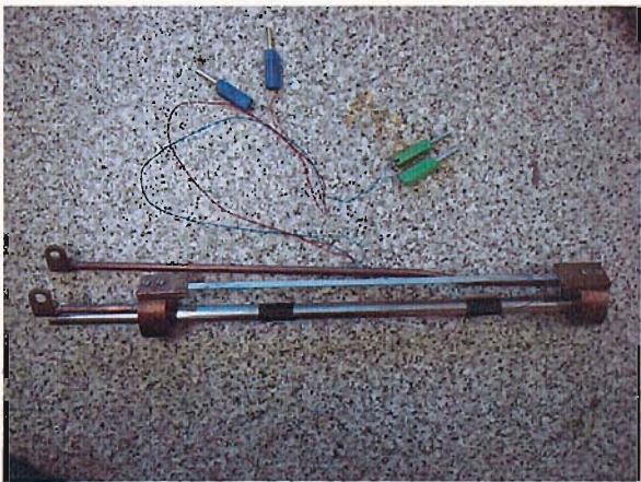
Figure 3.21. Rig for the HTS element testing
