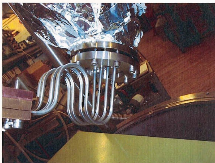
Figure 4.18. The current lead assembly enters from the bottom flange of the LHe vessel
