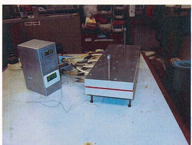
Figure 3.21. Aluminium plates for brazing the HTSC boards and the temperature controller
