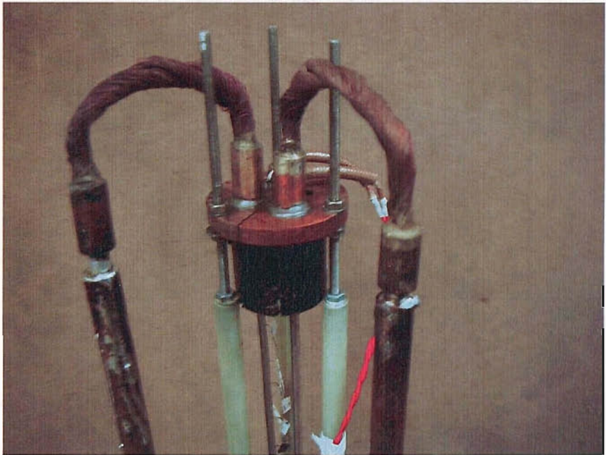
Figure 5.4. The connections of the current leads to the top copper block
