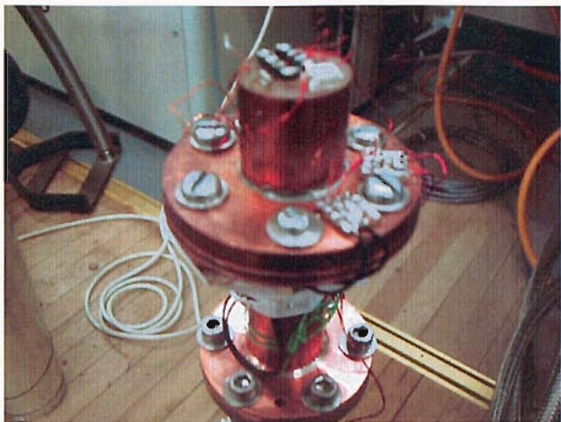
Figure 3.27. Rig for electrical resistivity measurements
