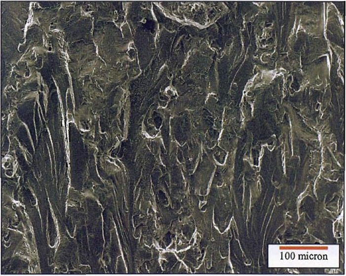
Figure 4.16 Fracture surfaces observed at \Delta K \sim 9 \text{ MPa}\sqrt{\text{m}} ; (a) 2027-ReX(8), (b) 2027-ReX(55), and (c) 2027-ReX(100).
