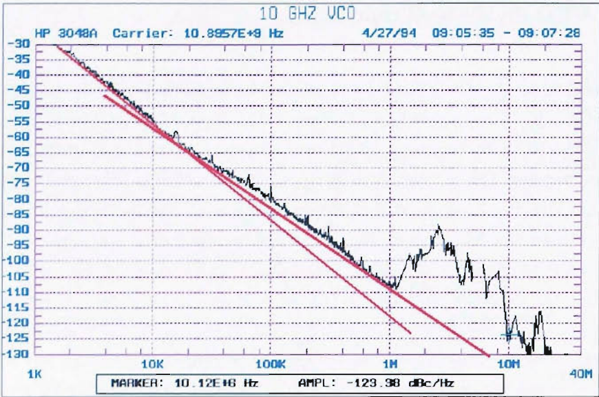
FIGURE 6.33: Measured phase noise of the VCO output (no divide-by-2) using the HP3048A phase noise system together with a high frequency probe station.
