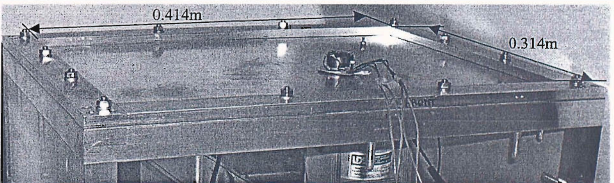
Figure 4.7: Photography of the experimental set-up with the primary shaker below the plate in the background and the inertial actuator above the plate in the foreground.
