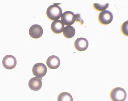
Figure 4.8 Photograph of selectively stained beads after treatment with 0.1 mM CuCl 2 and dithio-oxamide.
