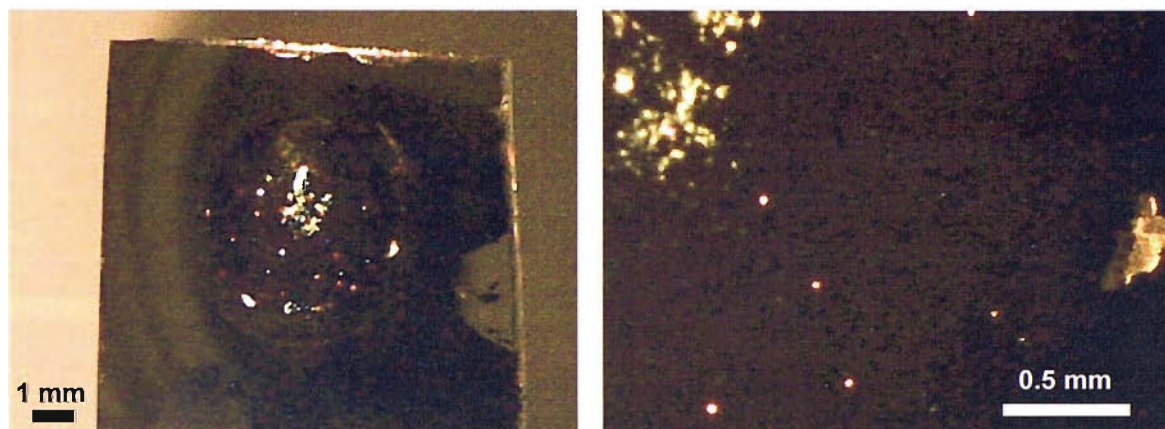
Figure 31. Evaporated nickel slide with structured gold deposit of 5.7 mm (defined by masking with nail polish prior to gold deposition) diameter and 2.5 \mu\text{m} thickness. Structure was 5 \mu\text{m} diameter cavities. Taken with an Intel Digital Blue™ QX3+ microscope.
