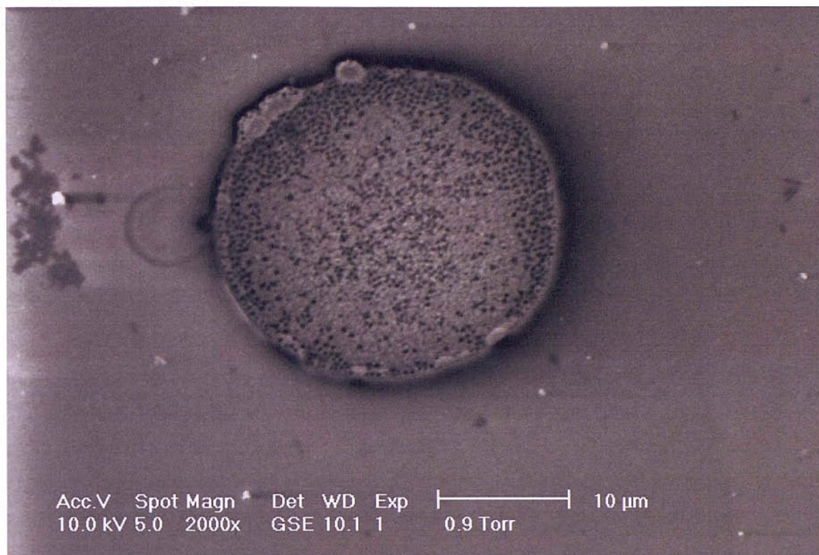
Figure 24. ESEM images of a 25 µm platinum disc recessed by ~ 1.85 µm. After electrophoretic assembly of 500 nm polystyrene latex; deposition of gold (charge passed = 2.8 µC) and soaking in THF (15 min). Taken with a Philips XL30 ESEM.
