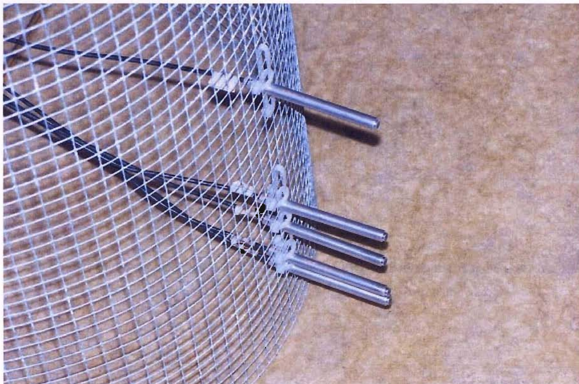
FIG. 6.1B: A wire-mesh used as a microphone holder for a normal-incidence measurement
