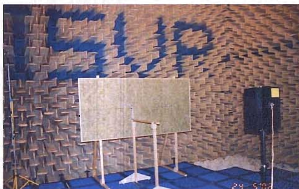
FIG. III.10: First measurement setup for normal incidence measurement in a free field.
