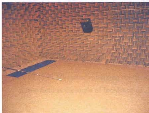
FIG. III.18-B: Free-field measurements in an anechoic chamber
