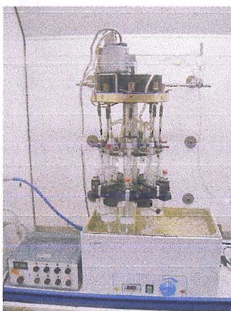
Figure 2.11: Suspension polymerisation reactor, internal volume 500 mL.
