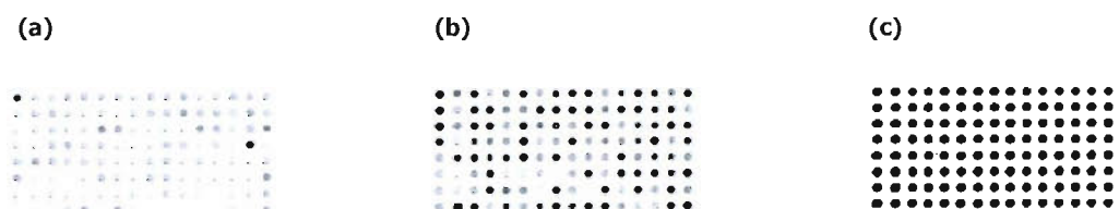
Figure 4.38 show three arrays spotted with 100 nM Cy3 labelled probe by the same pen.
