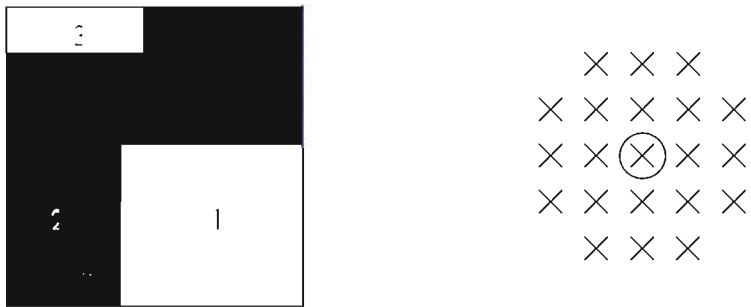
Figure 3.10: A 7 \times 7 mask window with the number of connected regions more than two. Therefore, the medium mask size is used.
