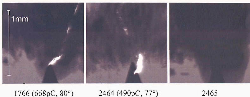
Figure 5.12, Selected images showing negative tip filamentary discharge recorded at 5000 fps, 1.24 mm frame width at 26.4 \pm 0.4 kV, 75.7 \pm 0.5 K
