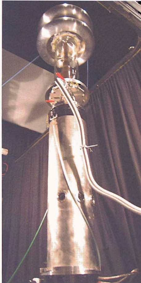
Figure 3.5, Cryostat with bushing
