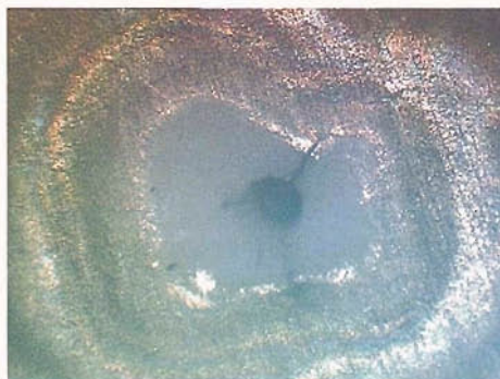
Figure 6.15, PTFE puncture from breakdown
