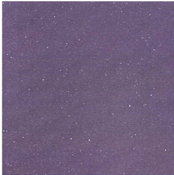
FIGURE 4.4: The dark image obtained with a 100 sec exposure at 20 °C.
