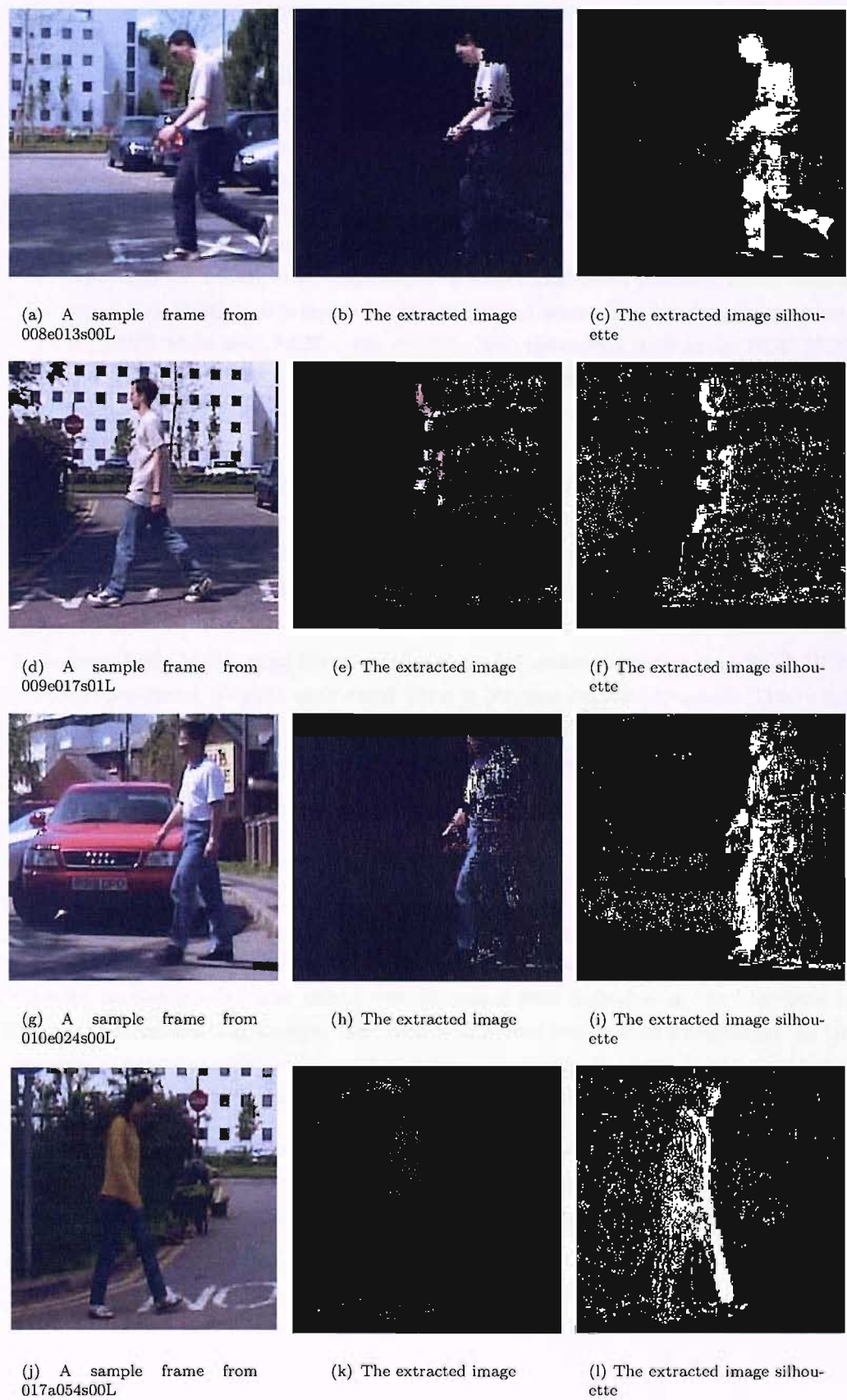
FIGURE 5.7: Examples of outdoor images extracted using the MOG algorithm with the c_1c_2c_3 colour model.
